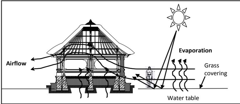
Figure 5: Creating comfortable Internal Environment
