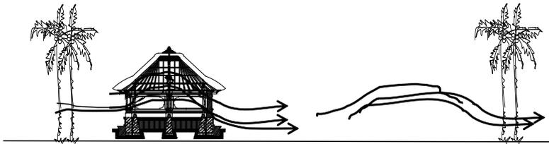
**Figure 4:** Cross ventilation at night and mid day easily occurs
