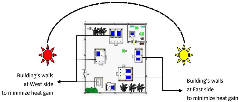
**Figure 3:** The positions of building wall to protect indoor comfort from solar heat
